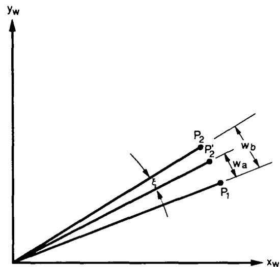
Figure 15.—Orientation of concave and convex sides of gear-tooth surfaces to attain proper top level width by rotation of convex side of tooth:  $P_1$ , concave side location of face angle point at toe end of tooth;  $P_2$  and  $P_2'$ , initial and final convex side locations, respectively, of face angle point at toe end of tooth;  $\xi$ , angle through which  $P_2$  is rotated; and  $w_b$  and  $w_a$ , desired and initial top level thicknesses, respectively.
