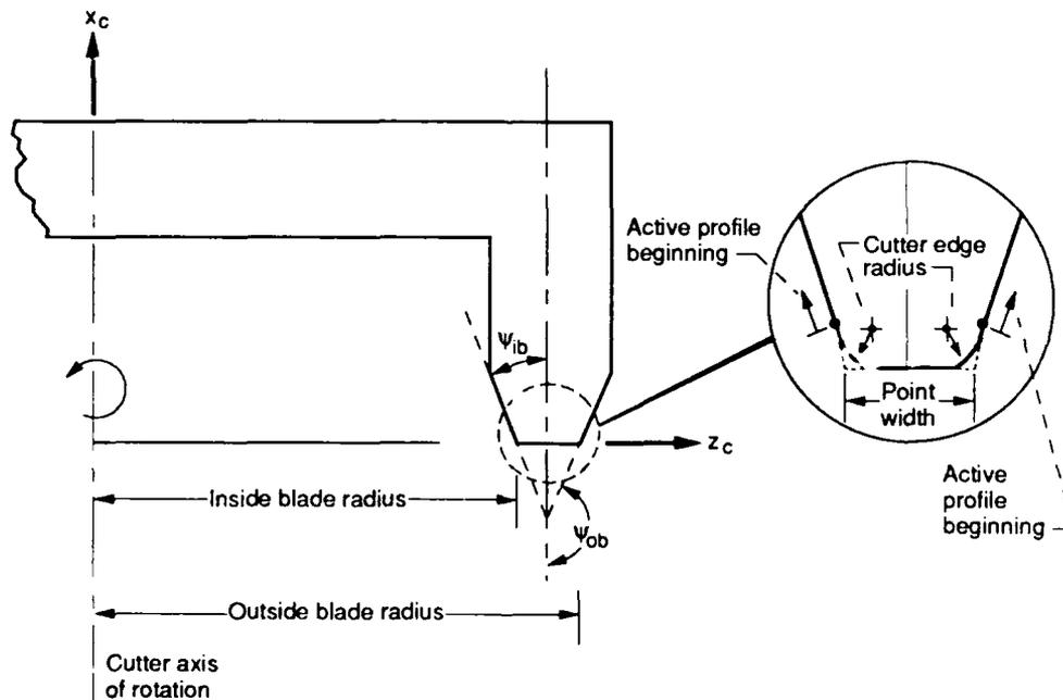
Figure 13. Detailed view of straight sided cutter geometry
