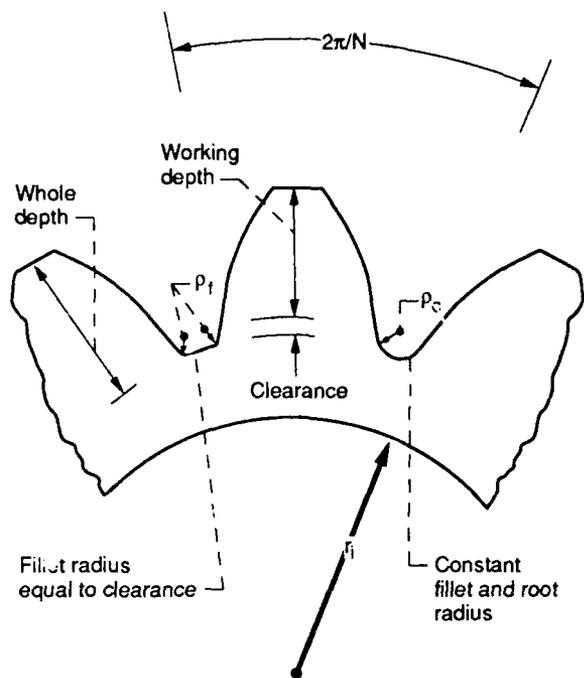
Figure 14.—Two types of fillet and root radius regions used by SURFACE program:  $\rho_c$ , constant fillet and root radius;  $\rho_f$ , fillet radius equal to the clearance;  $N$ , number of teeth;  $r_i$ , inside radius of gear blank.
