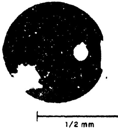
Fig. 2. An active fallout particle from a tower shot in Nevada. The particle is spherical with a brilliant, glossy surface.
