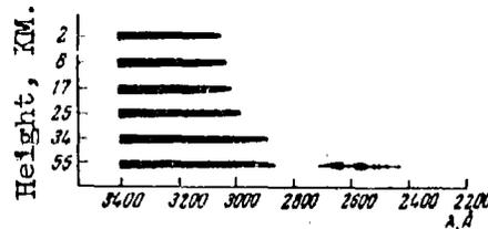
Fig. 1. Spectrograms obtained during flight of rocket (Kondrat'yev, 1954).
