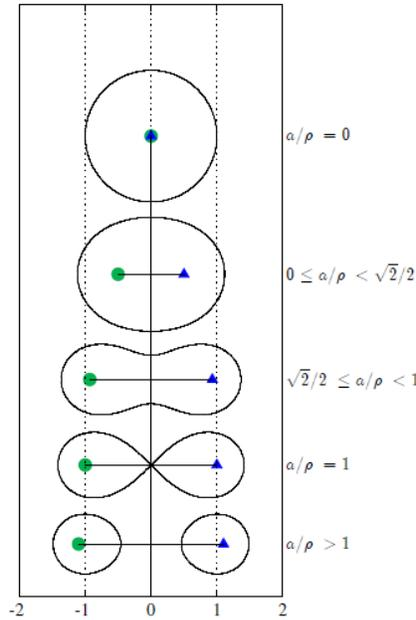
Figure 2. Cassini ovals corresponding to various values of  $a/\rho$ . Receivers and sources are denoted by # and • symbols respectively. For  $a/\rho = 0$  the oval is a circle. For  $a/\rho < \sqrt{2}/2$  the curve is a single loop. For  $\sqrt{2}/2 \leq a/\rho < 1$  the oval attains a dent on top and bottom. When  $a/\rho = 1$  the curve is a lemniscate. For  $a/\rho > 1$  the curve splits into two ovals (Karataş, 2013; Karataş and Akman, 2015).
