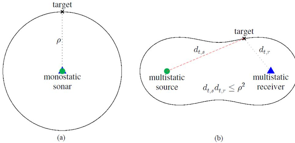
Figure 1. (a): Monostatic sensor with a disk shaped detection region of radius  $\rho$ . (b): Multistatic source and receiver detecting targets inside the region satisfying  $d_{t,s}d_{t,r} \leq \rho^2$ . Targets, receivers, and sources are denoted by  $\times$ ,  $\#$ ,  $\bullet$  symbols respectively.
