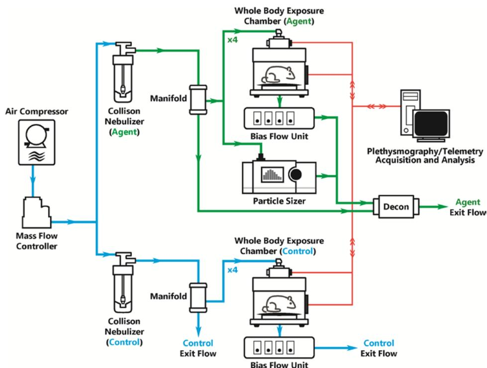
Figure 1. Configuration of CRF inhalation exposure system.
