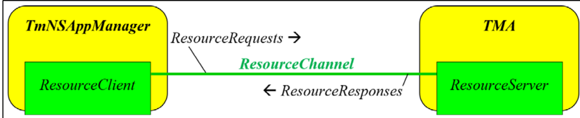
Figure 25-3. HTTP-Based Management Resources Channel Overview
