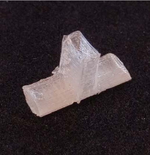
Figure 5: An SBS lens can be inserted into a piece of WR-28 waveguide to improve the antenna gain relative to open ended waveguide.
