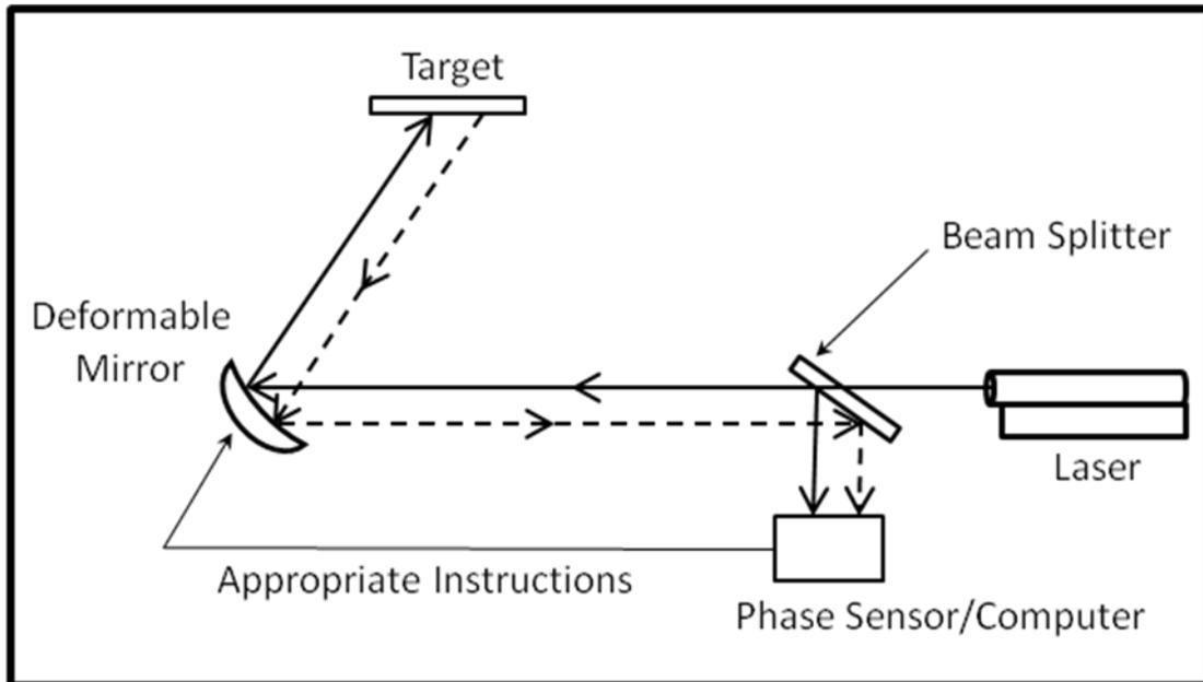
**Figure 3.** Schematic of an Adaptive Optics System
