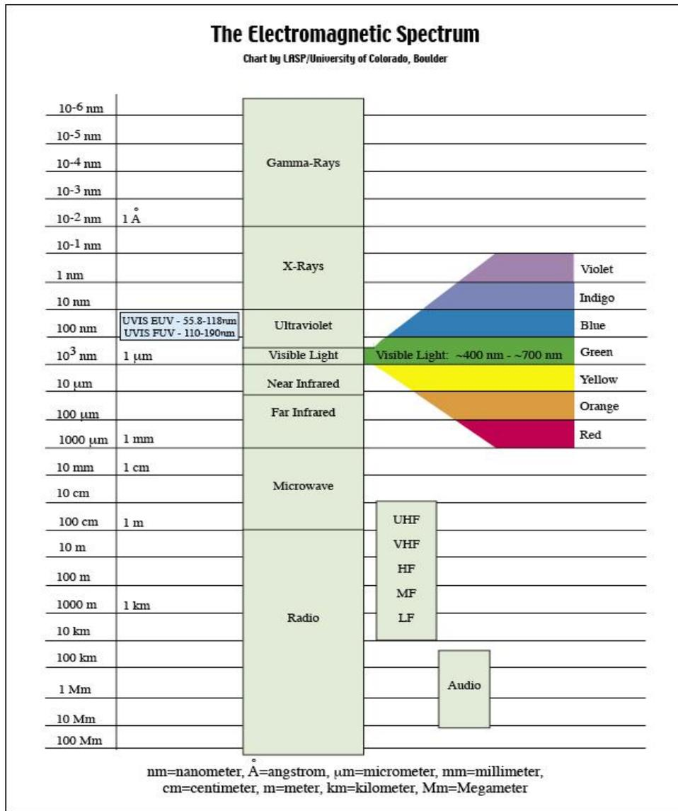
**Figure 1.** Electromagnetic Spectrum
