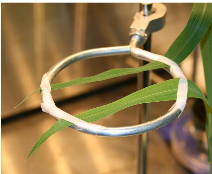
Figure 2. E. crus-galli leaf secured in horizontal position using tape folded in half lengthwise (to prevent leaf contact with the adhesive).
