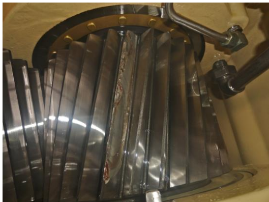
Figure 4. High speed pinion inspection result
